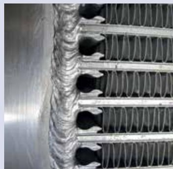
Classic Series uses patented AKG profiles to reduce local peak strains. This way, the strength of heat exchangers is significantly increased and their service life time considerably prolonged.
