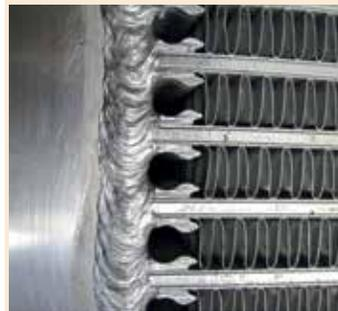
Cool-Line uses patented AKG hollow profiles to reduce local peak strains. This way the strength of heat exchangers is significantly increased and their service life time considerably prolonged.
